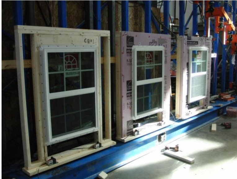
FIGURE 2. LONG-TERM DEFLECTION UNDER SELF-WEIGHT TESTING
