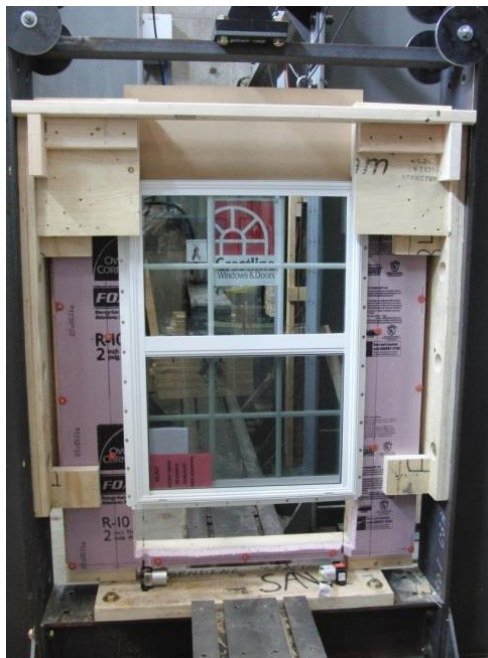
FIGURE 3. STRUCTURAL LOADING – FASTENER/FLANGE CAPACITY
