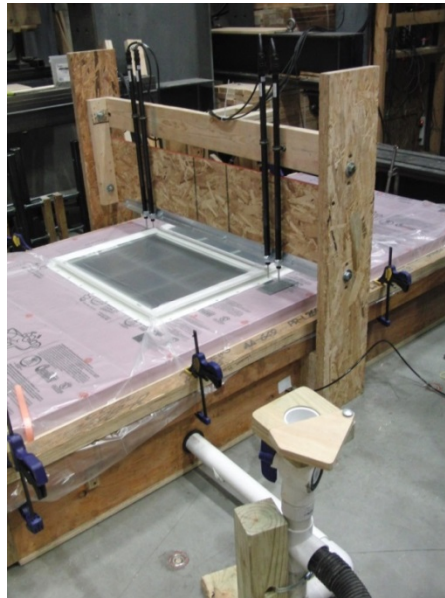
Photo 3: Wind Pressure Loading Test Setup
