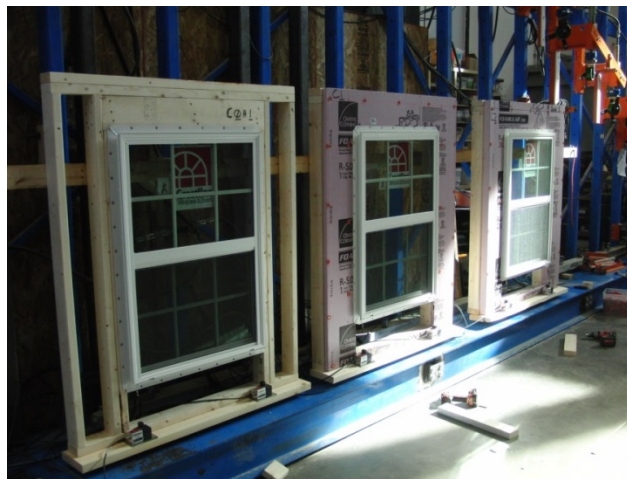
Photo 1: Long-Term Deflection Under Self-Weight Testing
