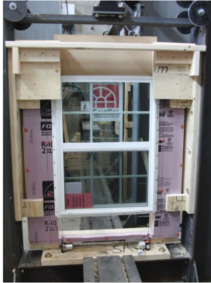
Photo 2: Structural Loading – Fastener/Flange Capacity
