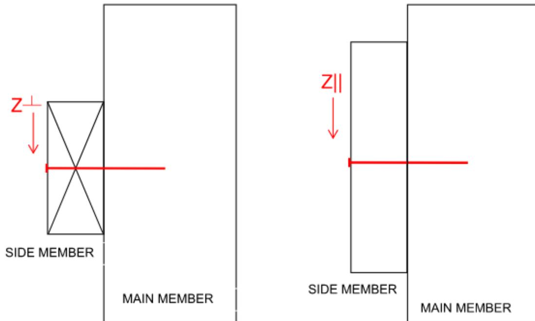
**Figure 6.** Lateral Load Directions
