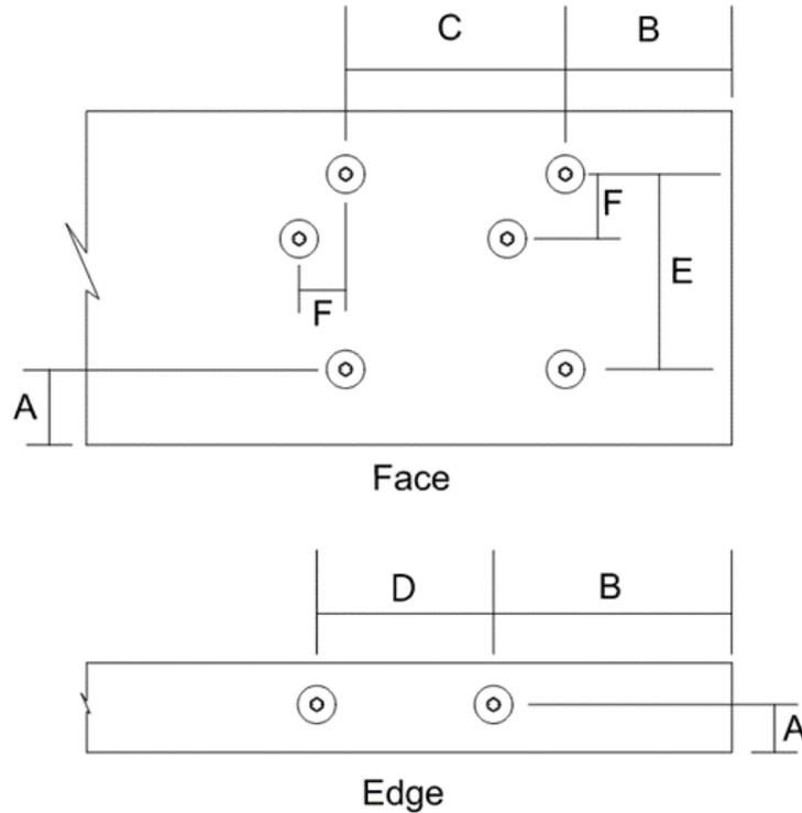
**Figure 7.** Fastener Spacing in Wood Reference Diagram
