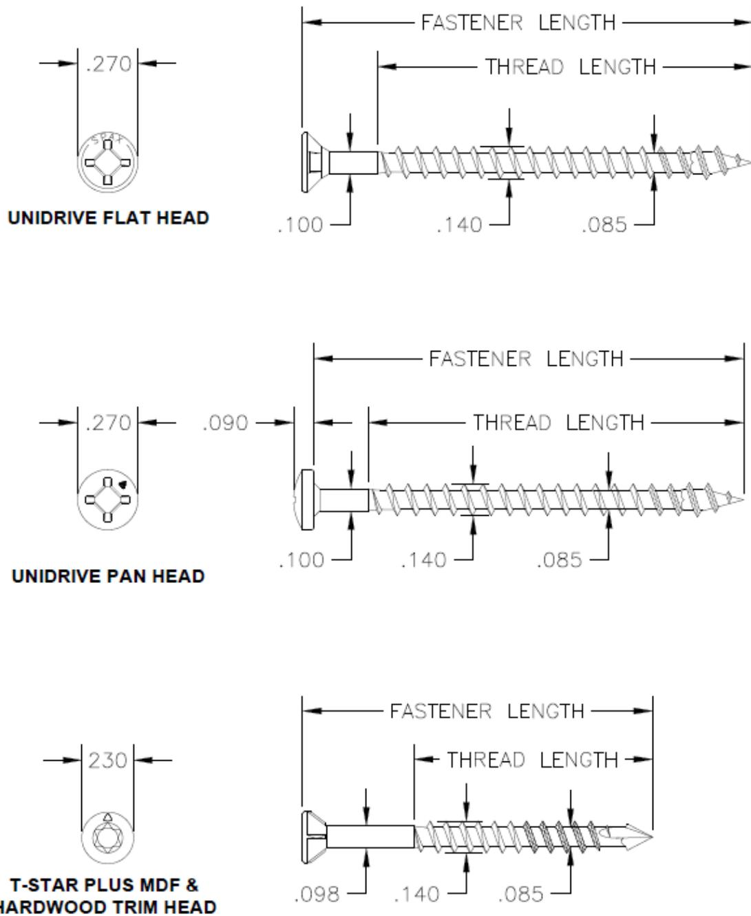
Figure 1. #6 SPAX® Construction Screws
