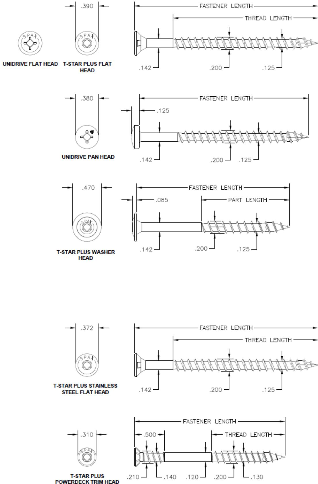
Figure 4. #10 SPAX® Construction Screws
