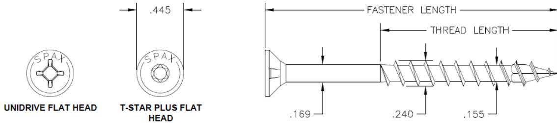
**Figure 5. #14 SPAX® Construction Screws**
